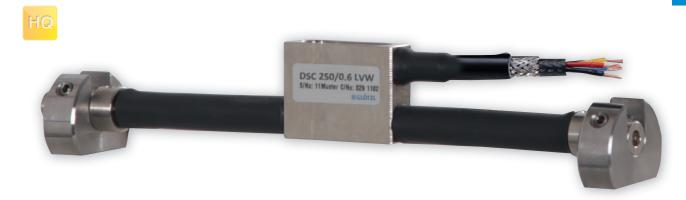
The vibrating wire strain gauge type DSC for arc welding to steel structures is commonly used for monitoring compression and/ or tension in struts (excavation bracing), in structural members of buildings and bridges, girder constructions, sheet pile walls, tunnel linings and other steel structures.
